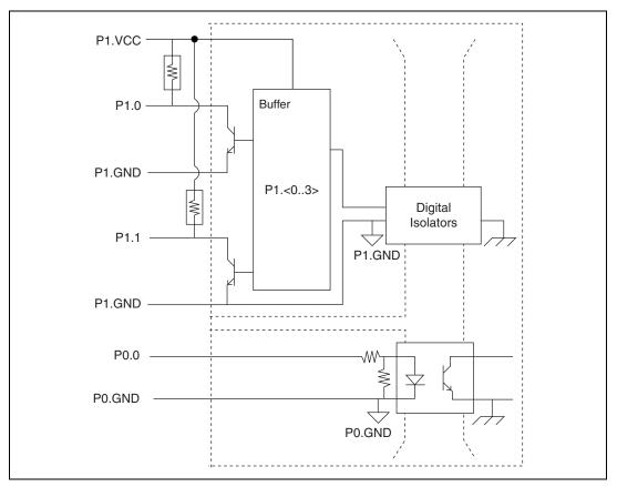
Figure 8-6. NI 6233 Digital I/O Connections (DO Sink)
